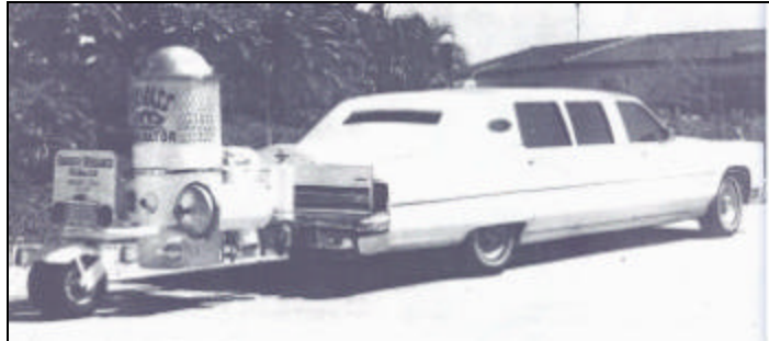
Car of yesteryear powered by Wood based Producer Gas (6)
