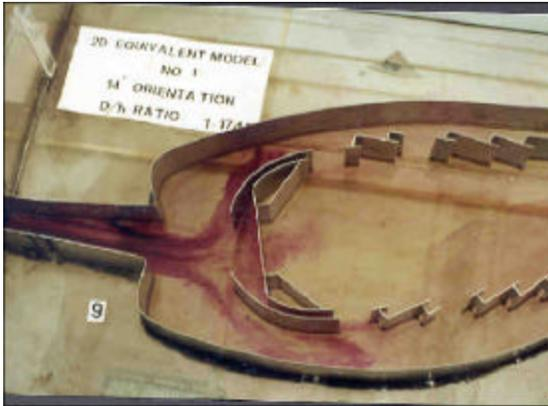
**Fig. 5 Dye Flow Pattern inside the 2-D Combustor Model**
