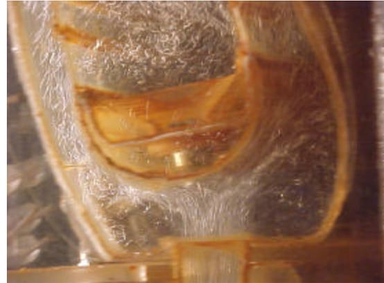
**Fig. 6 Flow Pattern Observed In the Dump Region Medium Water, Tracer-Air Bubbles,  $Re-10^5$**
